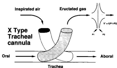
**Fig 1.** Experimental set-up showing the design of the tracheal X type cannula allowing simultaneous breathing and sampling of the eructated gas. The proximal end of the cannula is connected to a pneumotachograph, an airflow measuring device based on the use of the Venturi principle. The flow of air is proportional to the pressure difference on both side of a capillary grid which induces a small resistance.
