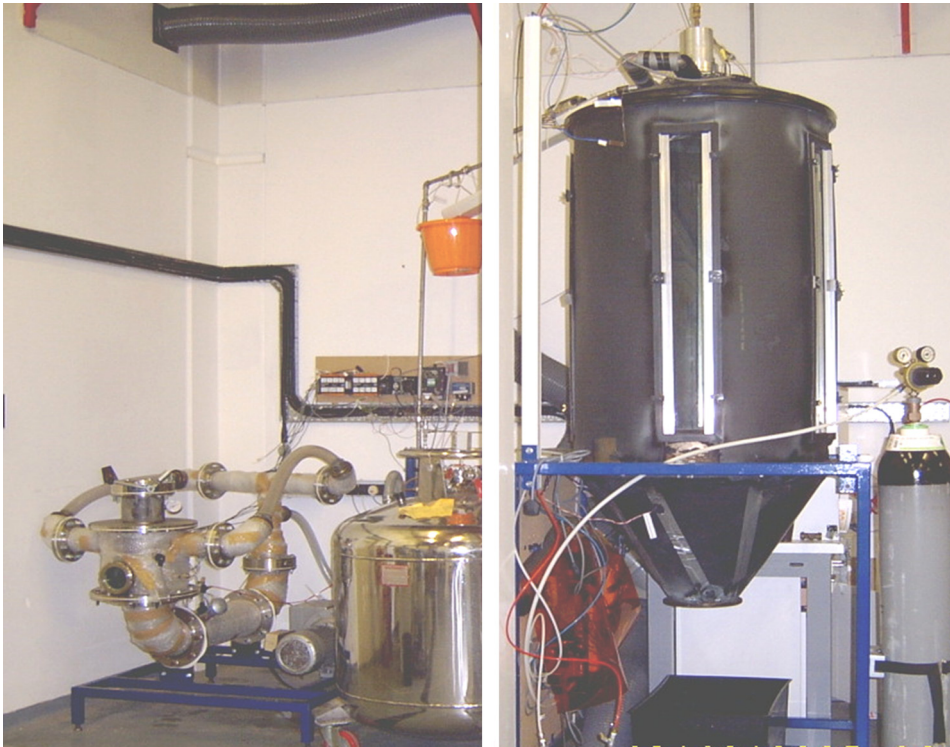
Figure 1. The SFD apparatus used in these experiments. Spray-freezing initially occurs in the large (black) chamber located on the right of the photograph. The spray frozen particles are collected from the base of this chamber and transferred to the sub-atmospheric fluidized bed freeze-drying apparatus on the left of the photograph.
