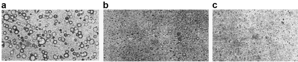
Figure 3. Micrographs of milk samples: (a) without homogenization (average size of fat globules \sim 4\text{--}7\ \mu\text{m} ), (b) ultrasonic homogenization at 90 W for 10 min (average size of fat globules \sim 2\ \mu\text{m} ) and (c) ultrasonic homogenization at 450 W for 5 min (average size of fat globules < 1\ \mu\text{m} ). (Adapted from Figure 1 of [33].)
