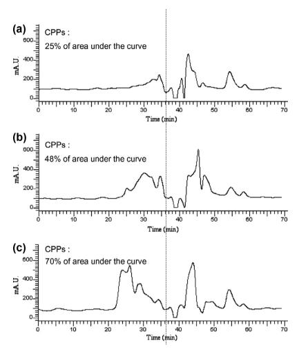
**Figure 3.** Analysis of IMAC fractions III (a), IV (b) and V (c) obtained on calibrated Superdex<sup>®</sup> Peptide gel filtration chromatography column. Fractions I and II are not shown because no significant amounts of molecules eluted before 36 min (i.e. having a molecular weight  $> 600 \text{ g} \cdot \text{mol}^{-1}$ ) were present. mAU stands for milliunits of absorbance at 215 nm.
