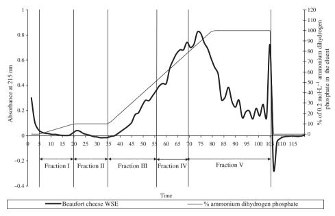
**Figure 1.** Chromatogram of Beaufort cheese WSE on the IMAC column, and separation into fractions according to Lund and Ardö [14]. The column was eluted with a gradient of 0 to 0.2 mol·L<sup>-1</sup> ammonium dihydrogen phosphate pH 4.4. Detection was performed at 215 nm. Total loaded samples correspond to 1.5 g Beaufort cheese.
