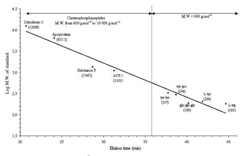
**Figure 2.** Calibration of Superdex® Peptide PE 7.5/300 GFC column using standard peptides. The elution was carried out with 30% of 0.1% TFA in acetonitrile and 70% of 0.1% TFA in water, with a flow rate of 0.25 mL·min<sup>-1</sup>. Detection was carried out at 215 nm.
