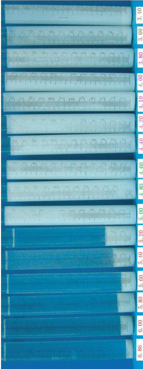
Figure 3. Visual appearance of phase behavior of acidified milk drinks at different pH values 15 days after preparation (the concentration of CMC ( M_w = 700,000 ) is 4 \text{ g}\cdot\text{kg}^{-1} ).
