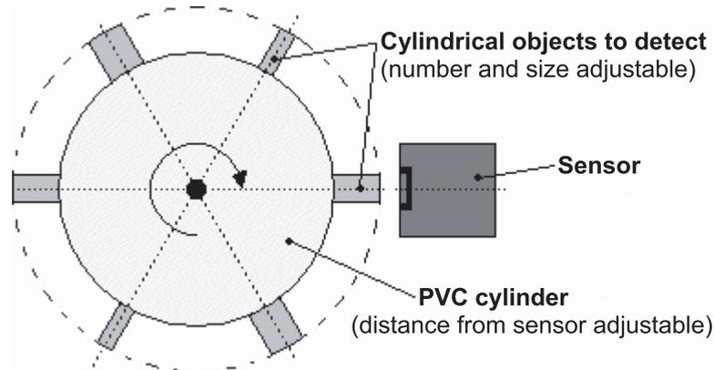
**Figure 2.** Experimental device used to validate the concept of the optical sensor.
