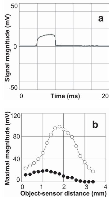
**Figure 4.** (a) Example of the pre-processed signal corresponding to the 1-cm PVC cylinder passing through the field of vision of the sensor in water; (b) Sensor response as a function of the distance of the object to detect in water (o) and whey (•).
