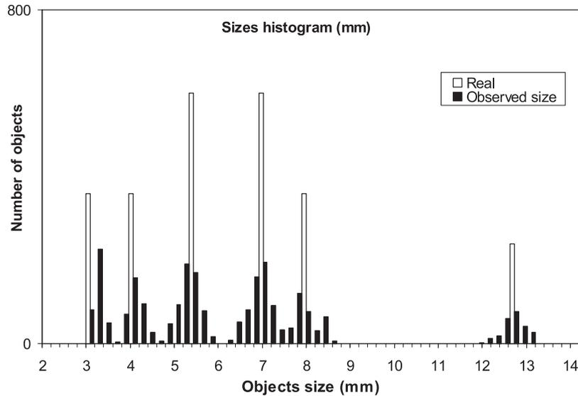
**Figure 5.** Histogram of measured (black) and real object (white) size when using experimental device in Figure 2. Object number and sizes are listed in Table I. The results were obtained by a simple threshold (10 mV) on the signal. The rotational speed of the PVC cylinder was 61 rpm.
