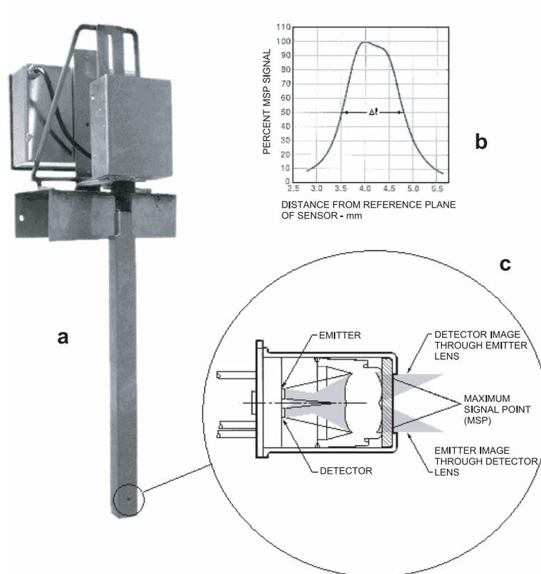
**Figure 1.** (a) General view of the sensor; (b) LED response in the air. Percentage of reflected signal relative to the signal level at the Maximum Signal Point (MSP) as a function of distance from reflector; (c) Transmitter-receiver diode cross-section.
