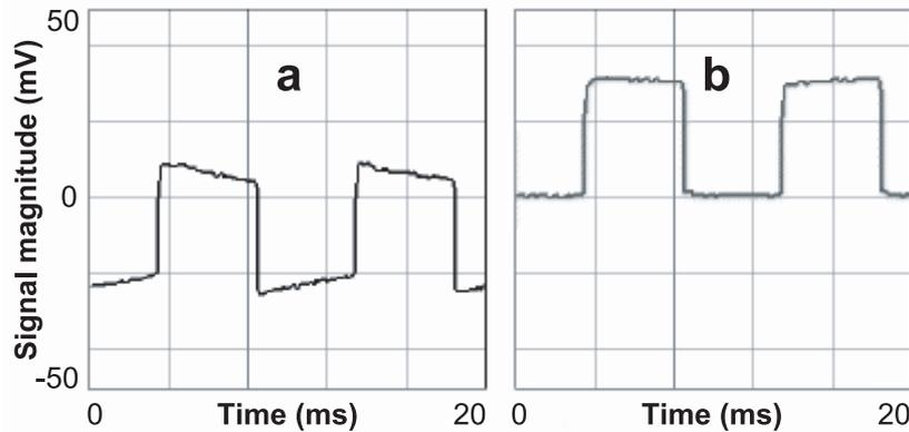
**Figure 3.** (a) Signal at the output of the DSP card without pre-processing when the input signal was a 30-mV magnitude rectangular signal, with a continuous offset of 15 mV, at 100 Hz frequency and a 50% cyclical ratio. The signal was deformed by the high-pass filter; (b) The same signal after pre-processed. The rectangular shape is recovered.
