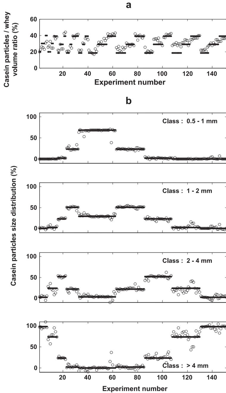
**Figure 6.** Estimation of the casein particles/whey volume ratio (a) and of the casein particle size distribution (b) using the optical signal-processing method based on neural networks. Application to 150 optical measurements not used for neural network calibration. Real (●) and estimated (○) values.
