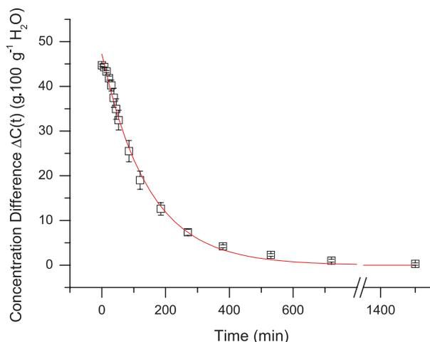
**Figure 3.** Concentration difference versus time. Typical graph of experimental data of seeded lactose crystallization from pure supersaturated solution at 30 °C (□) (initial lactose concentration of 70 g·100 g<sup>-1</sup> water). The curve represents the best first-order exponential decay fit.
