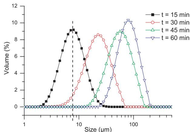
**Figure 4.** Crystal size distributions at different times during non-seeded lactose crystallization from pure supersaturated solution at 30 °C (initial lactose concentration of 70 g·100 g<sup>-1</sup> water).
