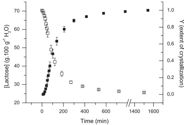
**Figure 2.** Desupersaturation curve ( $\square$ ) and extent of crystallization ( $\blacksquare$ ). Typical graph of experimental data of seeded lactose crystallization from pure supersaturated solution at 30 °C (initial lactose concentration of 70 g·100 g<sup>-1</sup> water).
