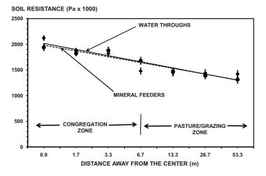
**Figure 4.** Regression analysis showing the relationship of soil penetrometer resistance with distance away from the center of the different congregation sites (solid line: water troughs = -112.8x + 2095.4;  $R^2 = 0.94^{**}$ ; dash line: mineral feeders = -119.5x + 2136.9;  $R^2 = 0.85^{**}$ ).
