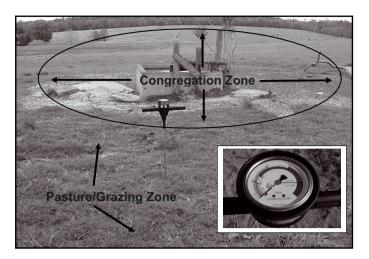
Figure 2. Taking measurements at congregation zone and pasture zone using a hand-held cone penetrometer (Dickey-John Corp).
