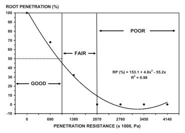
**Figure 6.** Relationship of root penetration (%) and soil penetrometer resistance (Pa) using hand-held penetrometer (Good root penetration:  $0 - 1.035 \times 1000$  Pa; Fair root penetration:  $1.035 \times 1000$  Pa -  $2.070 \times 1000$  Pa; Poor root penetration:  $> 2070 \times 1000$  Pa).
