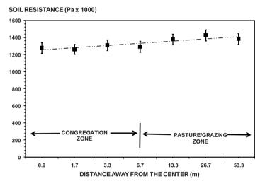
Figure 5. Regression analysis showing the relationship of soil penetrometer resistance with distance away from the center of shaded areas  $(25.6x + 1230.8; R^2 = 0.77^{**})$ .
