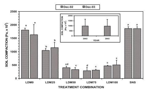
Figure 4. Degree of soil compaction for soils with varying levels of lake-dredged materials. Soil compactions from plots with or without lake-dredged materials are significantly different ( $P \le 0.05$ ) when superscripts located at top of bars are different.
