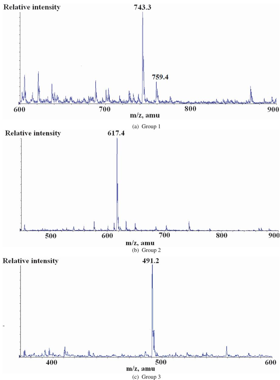
**Figure 3.** Electrospray ionization – mass spectrometric (ESI-MS) spectra of three isolates. 743.3, 617.6 and 491.2 are equal to the molecular weight of triesters, diesters and monoesters plus  $\text{Na}^+$ , respectively. This indicates the three compounds are mainly triesters, diesters and monoesters.
