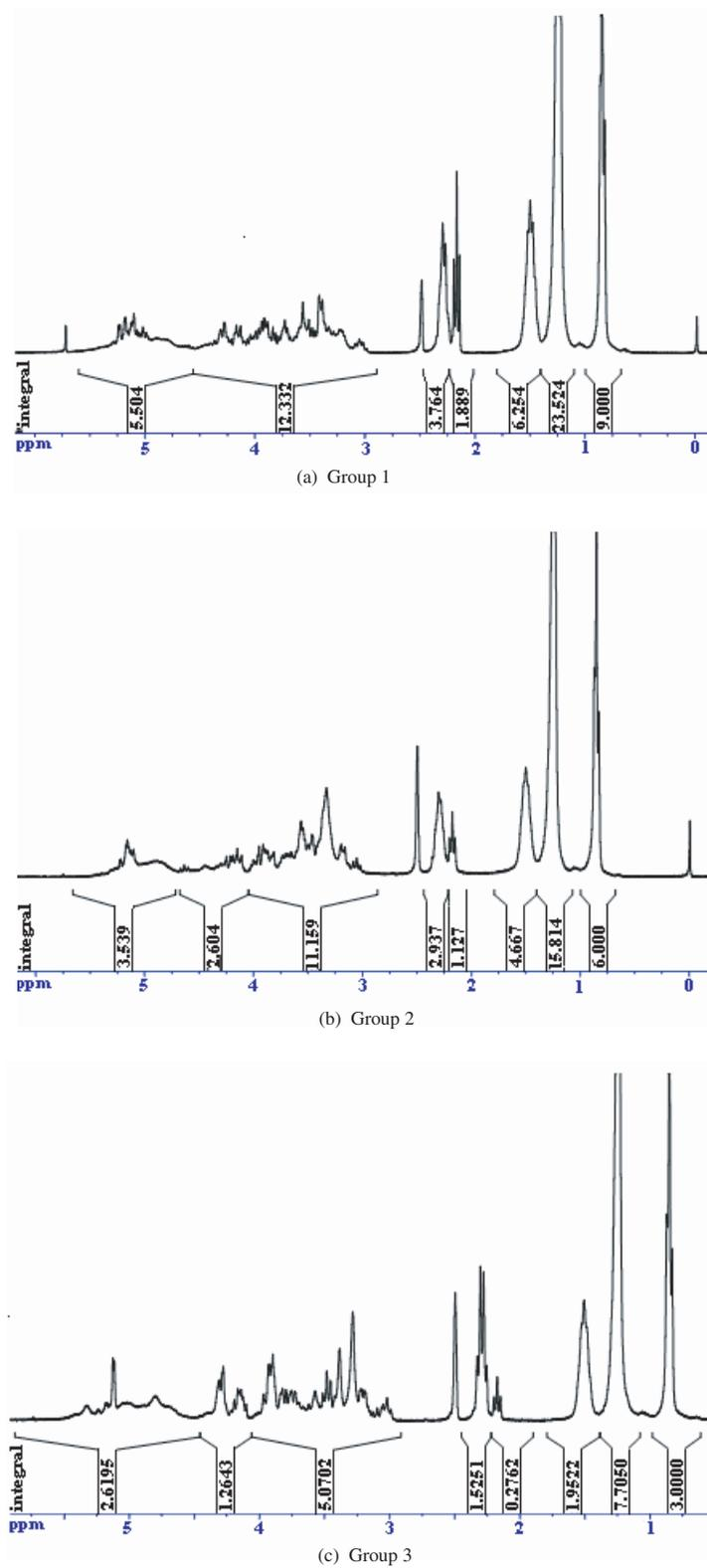
**Figure 4.**  $^1\text{H}$  nuclear magnetic resonance (NMR) spectrometric spectra of three isolates. According to the shift data and integral, Group 1 had three  $(\text{CH}_3\text{-(CH}_2)_5\text{-})$  groups and three  $(\text{-CH}_2\text{COO-})$  groups, Group 2 had two of both, and Group 3 had only one of each group. That suggests that the three compounds were triesters, diesters and monoesters, respectively.
