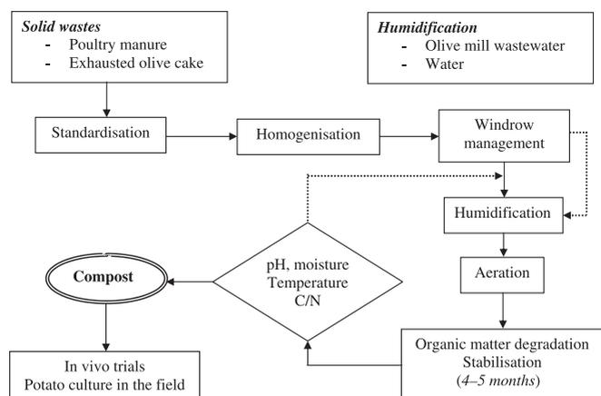
**Figure 1.** Experimental design and process controle. C: carbon content; N: total nitrogen content.
