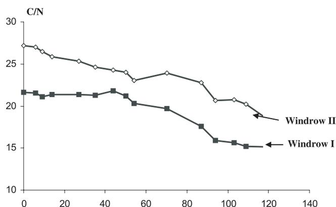
**Figure 3.** C/N ratio decrease during composting of mixtures of poultry manure and exhausted olive cake. Windrow I: 75% poultry manure and 25% exhausted olive cake; windrow II: 25% poultry manure and 75% exhausted olive cake.
