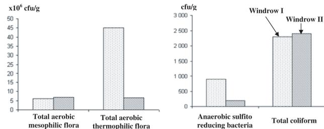
**Figure 4.** Microbial content of the mature composted windrows (cfu/g). Windrow I: 75% poultry manure and 25% exhausted olive cake; windrow II: 25% poultry manure and 75% exhausted olive cake.
