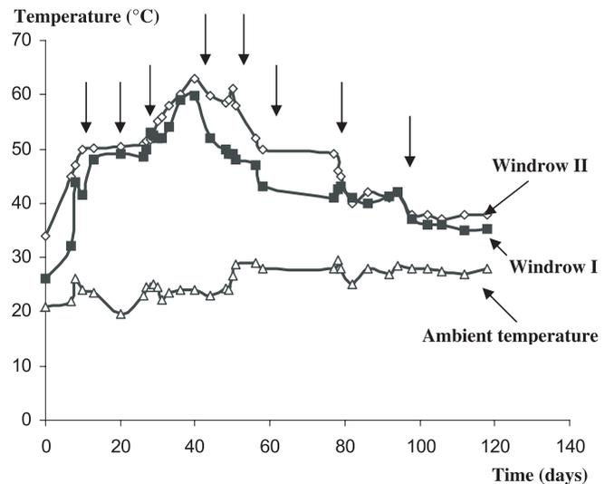
**Figure 2.** Temperature evolution during composting mixtures of poultry manure and exhausted olive cake. Windrow I: 75% poultry manure and 25% exhausted olive cake; windrow II: 25% poultry manure and 75% exhausted olive cake. Turnings are indicated by the arrows.
