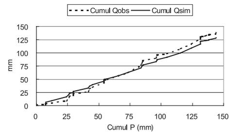
**Figure 7.** Double cumulative curves: cumulative simulated ( $\text{Cumul } Q_{sim}$ ) and observed ( $\text{Cumul } Q_{obs}$ ) drain flow rates and cumulative precipitation for intensive drainage season of Plot 6 ( $L = 5$  m), 1981–1982.
