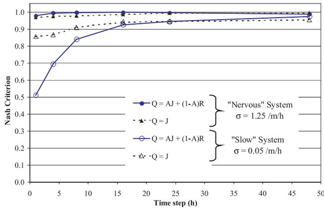
**Figure 1.** Nash's criterion versus time-step to compare the daily drain-flow rates between the two simplified models and the reference complete model in the case of a “nervous” system and a “slow” system.
