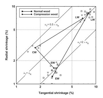
**Figure 5.** Radial shrinkage plotted versus tangential shrinkage for Douglas fir. Open marks represent individual measurements and plain marks average values per type of wood: earlywood (EW), compression wood (CW) and latewood (LW), see Figure 6.
