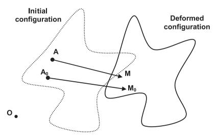
Figure 3. Notations used in the text to follow the materials points from the initial configuration (image of the saturated sample) to the deformed configuration (image of the air-dry sample).
