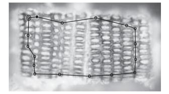
Figure 4. Example of two images (initial and deformed) and the corresponding chains of points plotted using the software *MeshPore* (Perré, [18]). This example corresponds to image 4 of spruce (late-wood).
