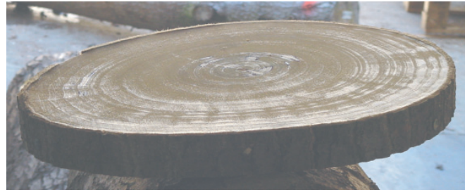
Figure 2. Tension wood areas from the cultivars MC viewed under a low angle natural light.
