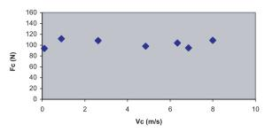
Figure 6. Cutting speed influence on cutting forces measured.
