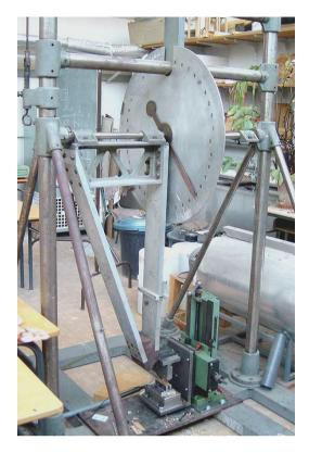
Figure 3. Dynamometric pendulum.
