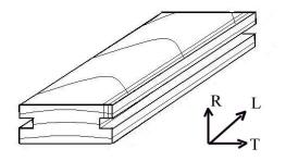
Figure 1. Wood specimen used for routing.
