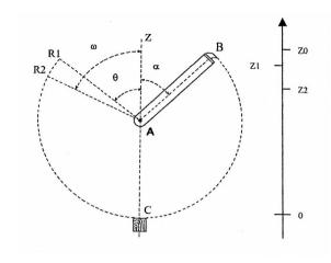
**Figure 5.** Use principle of dynamometric pendulum, where  $Z_0 = \operatorname{arm}$  starting height.  $Z_1 = \operatorname{arm}$  height after test without sample;  $Z_2 = \operatorname{arm}$  height after test with sample.
