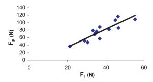
Figure 8. Relation between cutting forces obtained on router and on pendulum.
