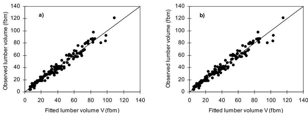
**Figure 5.** Observed (simulated using sawing simulator Optitek) lumber volume against predicted lumber volume in the case of the stud mill in jack pine. (a) Model 5 (second-order polynomial model with two variables “DBH and tree height”); (b) Model 6 (power model with two variables “DBH and tree height”).
