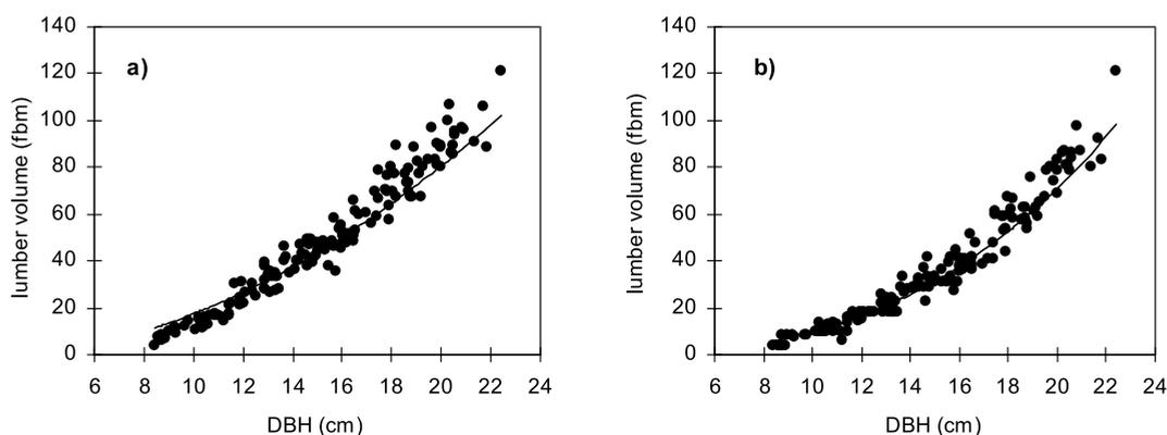
**Figure 6.** Predicted lumber volume recovery of jack pine for the stud mill in relation to DBH while holding tree height at an average level of 15.3 m. (a) Model 5 (second-order polynomial model with two variables “DBH and tree height”); (b) Model 6 (power model with two variables “DBH and tree height”).
