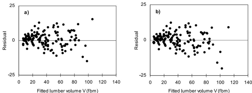
**Figure 3.** Plots of residuals against fitted lumber volume recovery in the case of the stud mill in jack pine. (a) Model 2 (second-order polynomial model with one variable “DBH”); (b) Model 3 (power model with one variable “DBH”).
