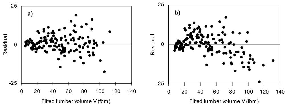
**Figure 2.** Plots of residuals against fitted lumber volume recovery in the case of the random mill in jack pine. (a) Model 2 (second-order polynomial model with one variable “DBH”); (b) Model 3 (power model with one variable “DBH”).
