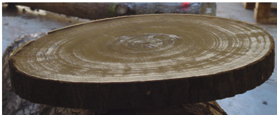
Figure 1. Tension wood areas from the Melone-Carlo cultivars viewed under a low-angle natural light.
