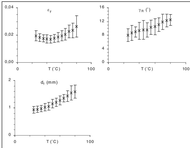
**Figure 8.** Evolution of  $\varepsilon_y$ ,  $\gamma_R$  (°) and  $d_f$  (mm) in function of temperature. Crosses represent the average value on ten wood species, vertical lines show the standard deviation.
