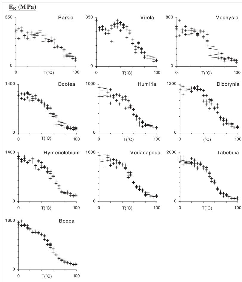
**Figure 9.** Evolution of  $E_R$  (MPa) from compression test in function of temperature for each wood species. Single cross represents one value of the three repetitions.
