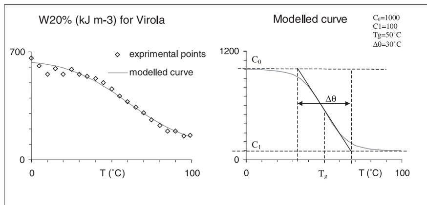
**Figure 7.** Illustration of the model of evolution of one criterion respect to temperature.
