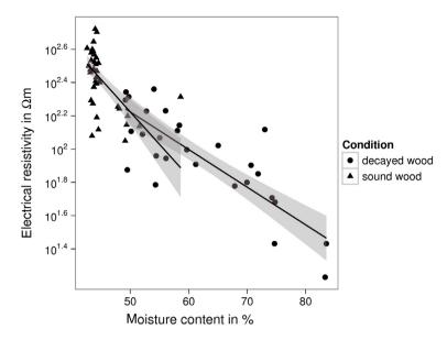
Figure 3. Electrical resistivity of tree No. 2 fell with increasing wood moisture content, which was significantly higher in decaying wood  $(R^2 = 0.79, p = 0.002)$ .
