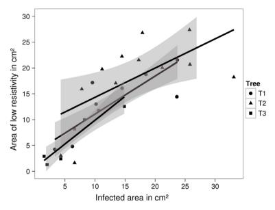
Figure 2. Area of low electrical resistivity against area infected by decay as detected visually in photos of stem cross-sections.
