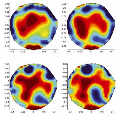
**Figure 4.** Tomograms of tree No. 3 made 10 cm above the dowels 3 (upper left), 10, 13 and 21 (lower right) month after infection with *Trametes versicolor*. Areas of low electric resistivity indicate increasing areas of infected wood. (A colour version of this figure is available at www. afs-journal.org.)
