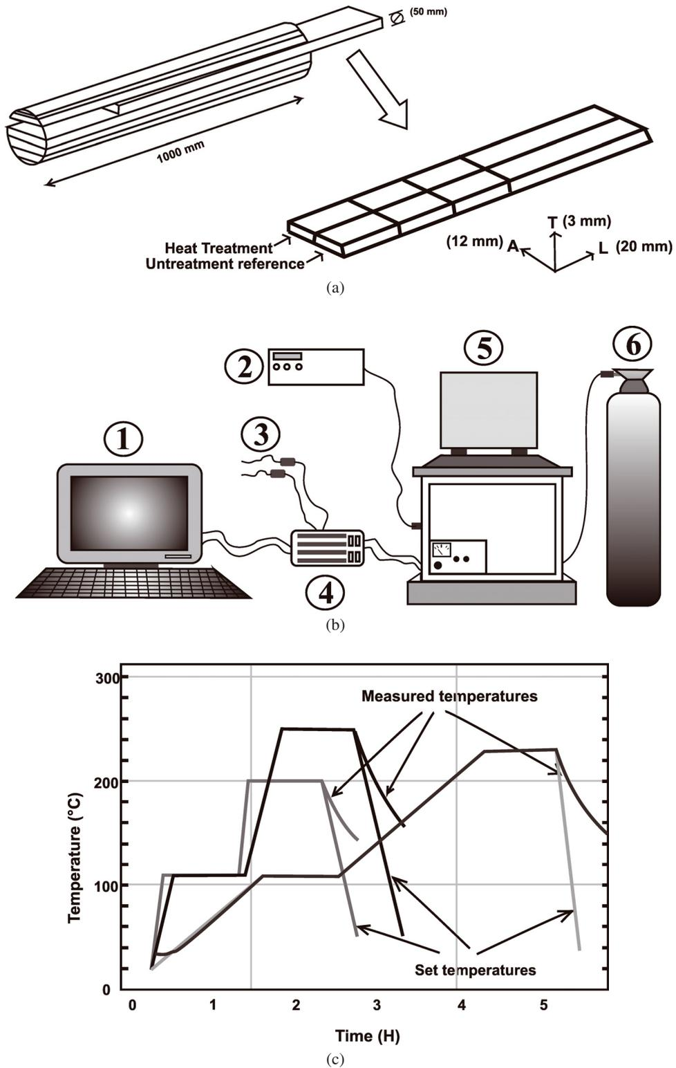
**Figure 2.** (a) Orientation and position of sampling from a board. (b) The experimental device used for thermal treatment: 1 – monitoring; 2 – O<sub>2</sub> analyser; 3 – probes; 4 – data capture; 5 – reactor; 6 – nitrogen. (c) Temperature evolution in the chamber during a typical heat treatment (set and measured temperature).
