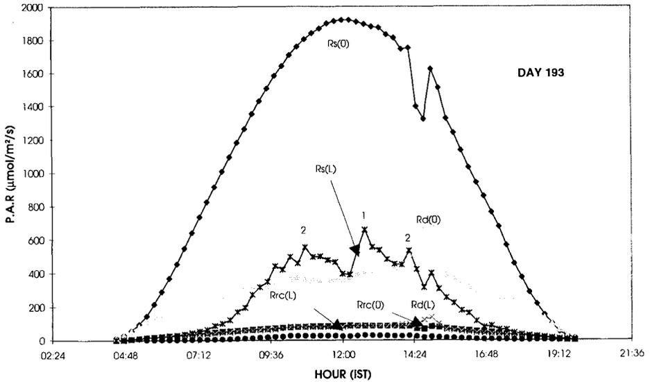
**Fig 1.** An example of PAR measurement on a sunny day, above and under the canopy. *Above the canopy:* PAR (global):  $R_s(0)$ ; sky diffuse PAR:  $R_d(0)$ ; PAR reflected:  $R_{rc}(0)$ . *Under the canopy:* PAR (global):  $R_s(L)$ ; understory diffuse PAR:  $R_d(L)$ ; PAR reflected by grass:  $R_{rc}(L)$ .
