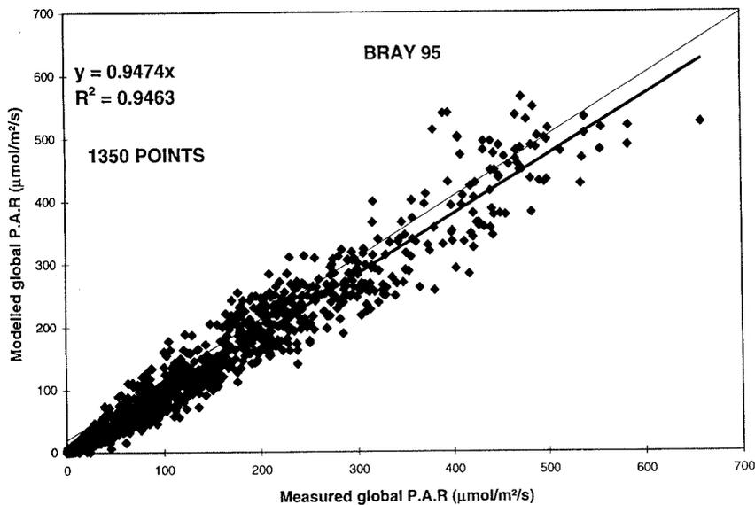
**Fig 10.** Comparison between modelled global PAR and measured global PAR by using all the data available between days 189 and 282. The values of the model are the sums of the estimated direct PAR and the estimated diffuse PAR.
