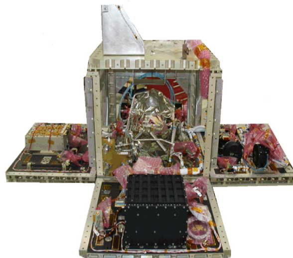
Fig. 9 MYRIADE platform example with the PICARD microsatellite.
