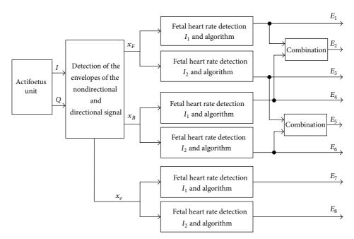
FIGURE 3: General diagram of the Doppler data processing acquired using one transducer and one channel.  $x_F$  and  $x_B$  represent the envelopes of the directional signals, and  $x_e$  represents the envelope of the nondirectional signal.  $I_1$ ,  $I_2$  are the two autocorrelation estimators.
