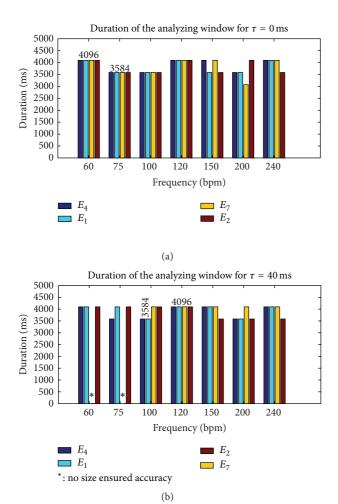
FIGURE 4: Duration of the analyzing window W required to reach an error of at least 0.25 bpm with the autocorrelation estimator  $(I_1)$  and a SNR > 0.6 dB.
