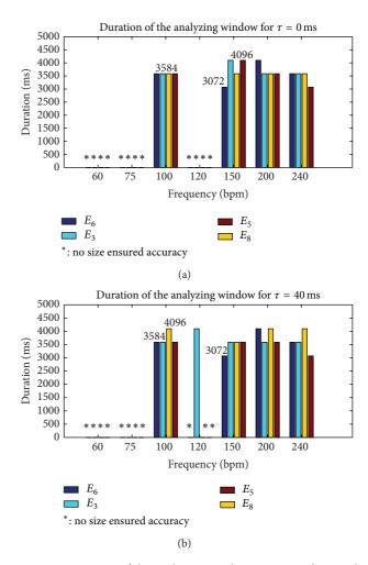
FIGURE 5: Duration of the analyzing window W required to reach an error of at least 0.25 bpm with the autocorrelation estimator  $(I_2)$  and with a SNR > 0.6 dB.
