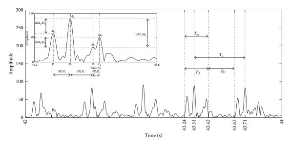
FIGURE 2: Envelope of a real directional Doppler signal of 2000 ms. The parameters defining the synthetic signal are the amplitudes and durations of peaks, the lag, and the differences in amplitude of two consecutive peaks over time.
