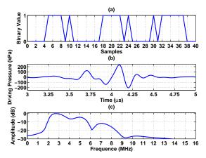
**Fig. 3.** (a) Optimal binary transmitted signal  $x_1(n)$  obtained by the genetic algorithm. (b) Signal p(n) at the transducer output (Fig. 1) when w(n) was the optimal binary signal and (c) its spectrum.
