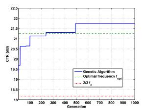
**Fig. 2**. Simulation of automatic optimization of the contrastto-tissue ratio (*CTR*) by a binary transmitted signal. The optimization was compared with the cases where the transmitted signal is at the optimal frequency and at the two-thirds of the central frequency of the transducer.
