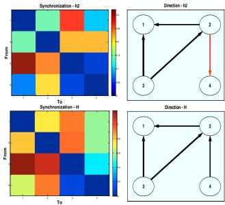
Fig. 2.Quantity (left) and direction (right) of information flow using Top: nonlinear correlation coefficient method  $(h^2)$  applied to the synthetic signal. The red arrow between nodes 2 and 4 indicates erroneous direction detection. Bottom: the index of general synchronization method (*H*) applied to the synthetic signal.
