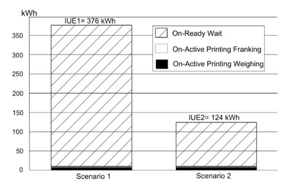
Figure 2: IUE results during planning showing the contribution of the functions.
