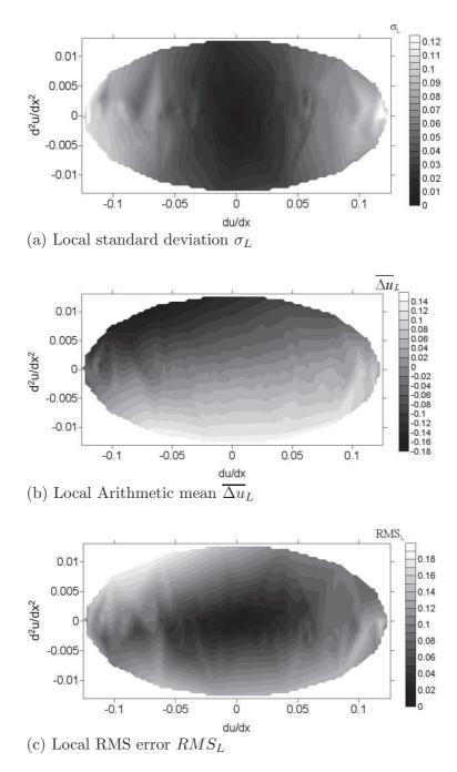
Figure 7: Influence of the first and second displacement gradients (d = 16 pixels, zero order shape function  $\Phi$ ).
