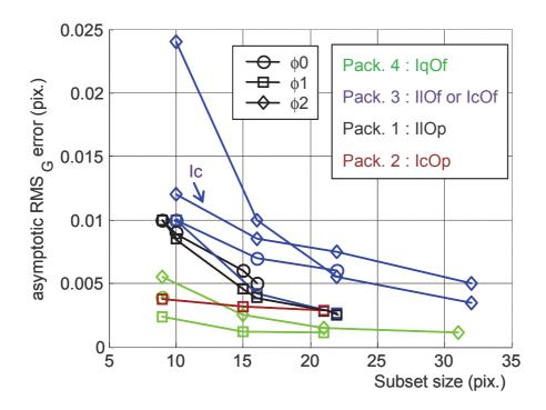
Figure 8: Comparison of the asymptotic RMS error  $\sigma^t(\phi, d, i, o, r)$  for quadratic, affine or rigid shape function and bilinear, bi-cubic or bi-quintic gray level interpolations as a function of the subset size. Speckle size is r = 2.2 pixels.
