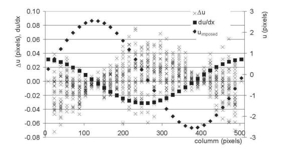
Figure 6: Imposed displacement, displacement gradient and local error  $\Delta u(i, j)$  as a function of the column of the image ( $\alpha = 0.005$ , p = 510 pixels, d = 16 pixels, zero order shape function  $\Phi$ ,  $u^{Max} = \alpha p = 2.55$  pixels, and  $\left(\frac{du}{dx}\right)^{Max} = u^{Max}_{,X} = 2\pi\alpha = 3.1\%$ ).
