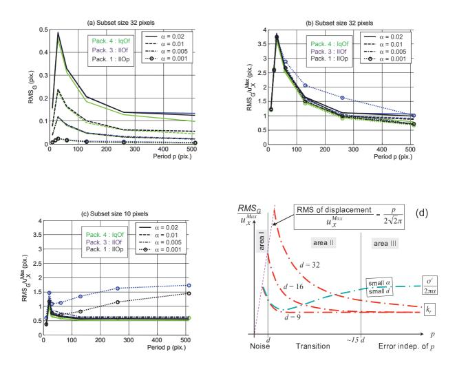
Figure 3: Evolutions of  $RMS_G$  with parameters p,  $\alpha$  and d, obtained with three packages implementing a zero order shape function and various gray level interpolations. Speckle size r = 2.2 pixels. (a)  $RMS_G$  as a function of p, subset size d = 32 pixels, (b)  $RMS_G/(2\pi\alpha)$  as a function of p, subset size d = 32 pixels, (c)  $RMS_G/(2\pi\alpha)$  as a function of p, subset size d = 10 pixels, (d) Schematic representation of all observations.
