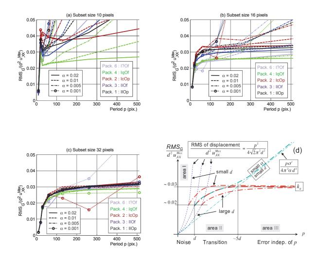
Figure 4:  $RMS_G$  normalized by  $4d^2\pi^2\alpha/p$  as a function of period p, for various strain amplitudes  $\alpha$ , for an affine shape function and for five DIC packages (20 curves). Subset size d is equal to 10, 16 and 32 pixels in plots (a), (b) and (c), respectively. (d) is a schematic representation of all observations.
