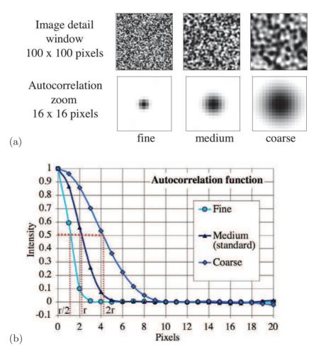
Figure 2: Illustration of synthetic speckle patterns. (a) fine, medium and coarse patterns and (b) associated centered and normalized autocorrelation function radius at half height.
