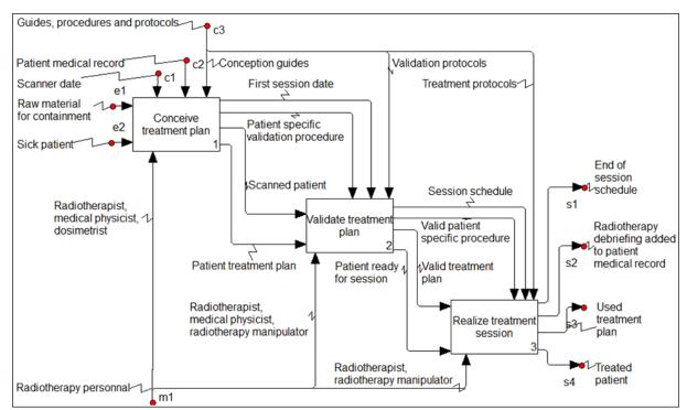
Figure 1. Highest decomposition level of the functional model of a radiotherapy treatment (SADT).
