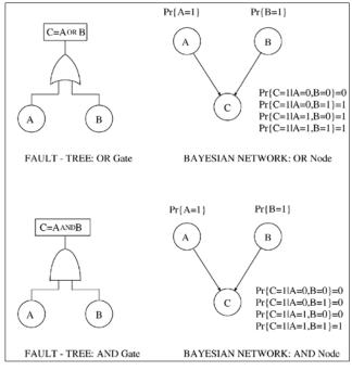
Figure 3. Equivalences between fault tree gates and Bayesian networks (Bobbio et al., 2001).
