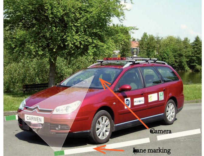
Fig. 5. Experimental vehicle. The camera is located behind the windshield.
