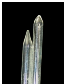
Fig. 8.8 Picture of a sonic probe (in the left) and of a glass finger with a thermocouple inside (in the right) used to sample species and measure the reaction temperature in the high pressure jet-stirred reactor used in Orléans (Dagaut et al. 1986)
