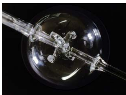
Fig. 8.2 Picture of the jet-stirred reactor used in Nancy (France) and which was developed from the rules of construction proposed by the group of professor Villiermaux
