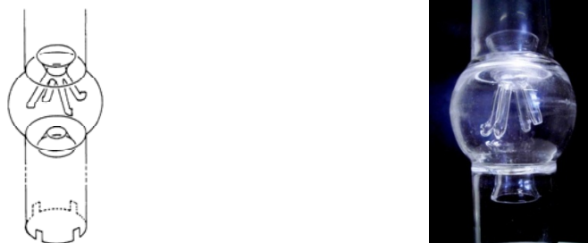
Fig. 8.6 Detail of the reactor developed in Orléans. The holes at the bottom of the prolongation tube are for pressure balancing
