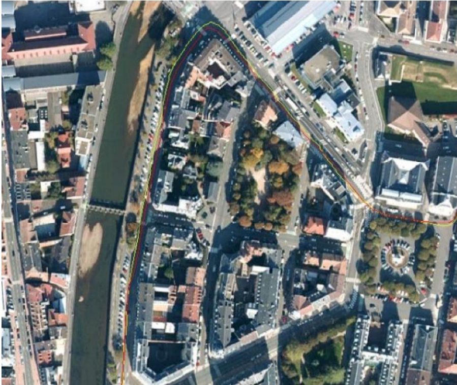
Fig 5: Example of one path of the vehicle in Belfort (the calculated position in yellow and the reference in red)
