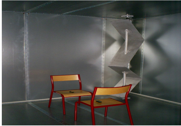
Figure 7: Inside view of the Reverberation Chamber in Université Paris-Est Marne-la-Vallée, LIGM, PasNet, France.
