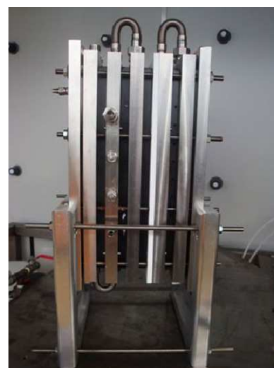
Fig. 3. Example of heat exchanger-reactor: reactor 4-mixed silicon carbide/stainless steel.
