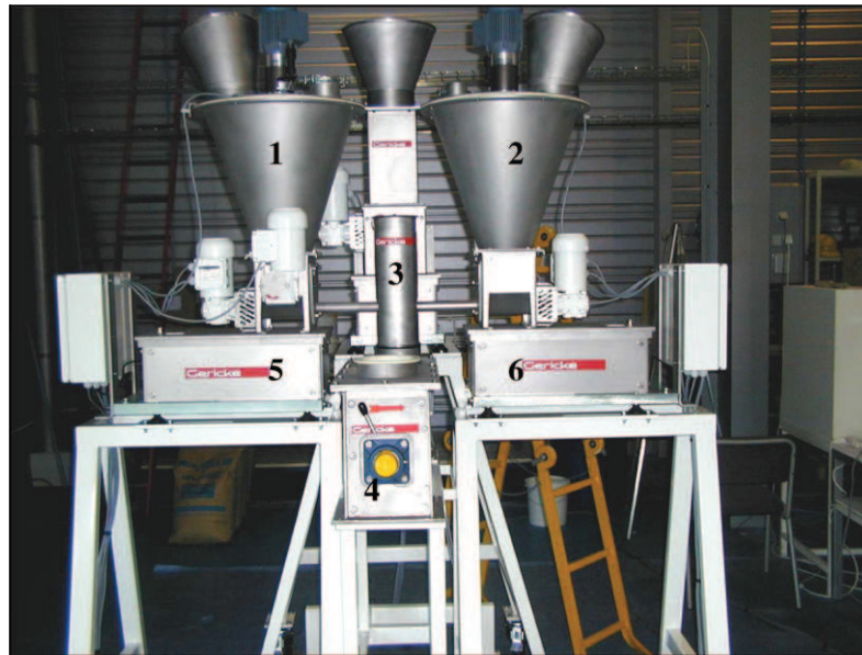
Fig. 2. Pilot scale continuous mixer Gericke GCM 500 used in the present work: loss-in-weight feeders (1,2); feeding chute tube (3); mixer outlet (4); balances (5,6).
