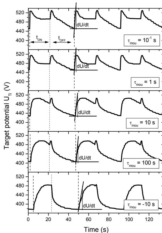
**Figure 3.10** Titanium target potential versus time for exponential patterns with various tau mounting times  $\tau_{\text{mou}}$ . The pulsing period was kept at  $T = 45$  s, the duty cycle  $\alpha = 0.444$  and the tau descending time  $\tau_{\text{des}} = 10^{-1}$  s. Derivative  $dU/dt$  was calculated at the beginning of each  $t_{\text{ON}}$  time in order to determine the speed of pollution of the target surface.
