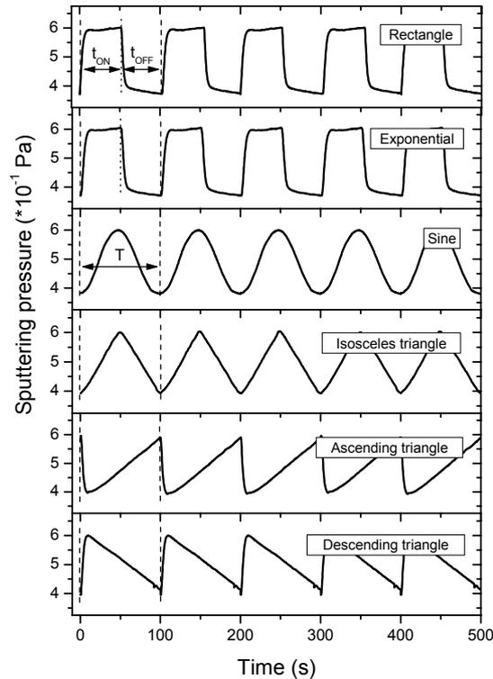
**Figure 3.4** Sputtering pressure versus time for all pulsing shapes and for a constant pulsing period  $T = 100$  s. For rectangular patterns,  $t_{ON} = t_{OFF} = 50\%$  of the pulsing period  $T$ . The same operating conditions were used for exponential signals with  $\tau_{mou} = \tau_{des} = 1$  s.
