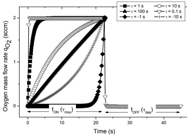
**Figure 3.8** Various shapes of signals can be generated with exponential pulses adjusting tau mounting time  $\tau_{mou}$  and tau descending time  $\tau_{des}$ . Tau descending time  $\tau_{des}$  is set to 0.1 s so as to stop the oxygen injection as similarly employed for rectangular pulses.
