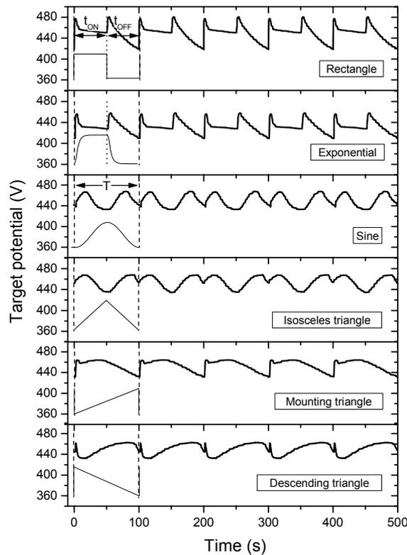
**Figure 3.5** Titanium target potential as a function of time for all pulsing shapes and for a constant pulsing period  $T = 100$  s. For rectangular patterns,  $t_{\text{ON}} = t_{\text{OFF}} = 50\%$  of the pulsing period  $T$ . The same operating conditions were used for exponential signals with  $\tau_{\text{mou}} = \tau_{\text{des}} = 1$  s.
