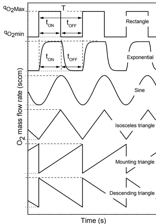
**Figure 3.1** Different periodic shapes of pulsing patterns of the oxygen mass flow rate versus time. Pulsing period  $T$ , injection times  $t_{ON}$  and  $t_{OFF}$  as well as maximal  $q_{O2Max}$  and minimal  $q_{O2min}$  oxygen mass flow rates can be controlled by RGPP.
