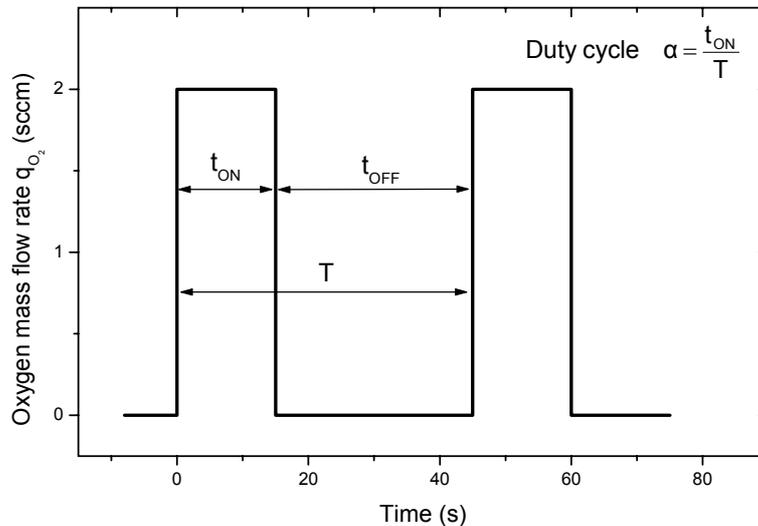
**Figure 3.6** Typical rectangular signals showing a schematic view of pulsed oxygen mass flow rate versus time with a pulsing period  $T = 45$  s and a duty cycle  $\alpha = 0.111$ , i.e.  $t_{ON} = 15$  s and  $t_{OFF} = 30$  s.
