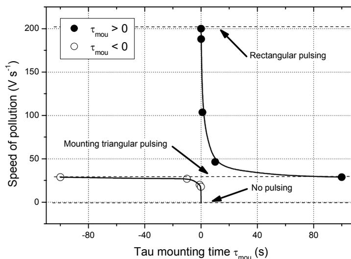
**Figure 3.11** Speed of pollution of the target surface versus  $\tau_{\text{mou}}$  time calculated from the time derivative of the target potential. Speed values obtained with rectangular ( $\tau_{\text{des}} = 0$  s) and mounting triangular pulses ( $\tau_{\text{mou}} \rightarrow +\infty$  or  $-\infty$ ) are given. No pulsing means no injection of the oxygen gas.
