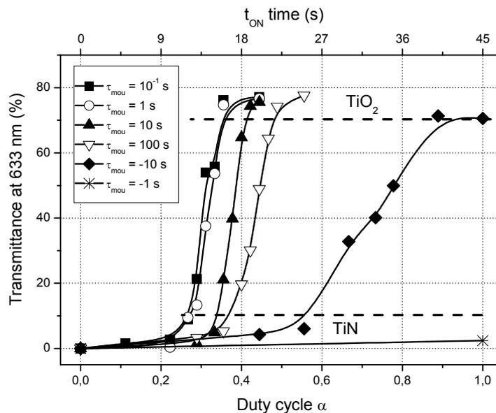
**Figure 3.9** Optical transmittance at 633 nm of titanium oxynitride thin films deposited on glass versus duty cycle  $\alpha$  and for  $\tau_{mou} = -10, -1, 10^{-1}, 1, 10$  and  $10^2$  s. The gradual transition zone from absorbent TiN to transparent  $\text{TiO}_2$  compound depends on duty cycle  $\alpha$  and tau mounting time  $\tau_{mou}$ .
