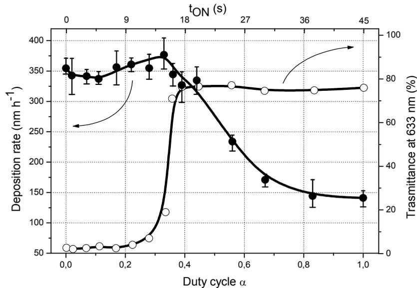
**Figure 3.7** Deposition rate and average optical transmittance at 633 nm of titanium oxynitride thin films sputter deposited on glass substrate as a function of the duty cycle  $\alpha$  and the corresponding  $t_{ON}$  oxygen injection time.
