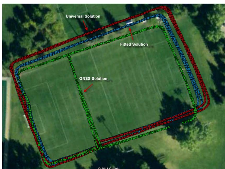
Figure 10. Reference path in green and estimated trajectories: modeled step length with the universal parameters in red and with the calibrated parameters in blue for the test subject with the worst performance (M5).
