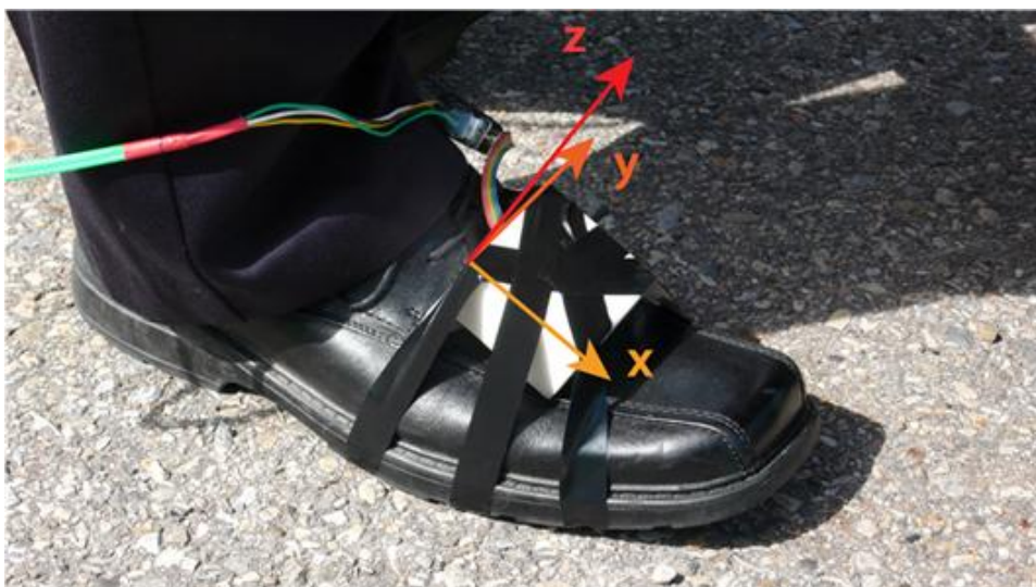
Figure 10. IMU attached on the foot and used as a reference for step detection assessment.
