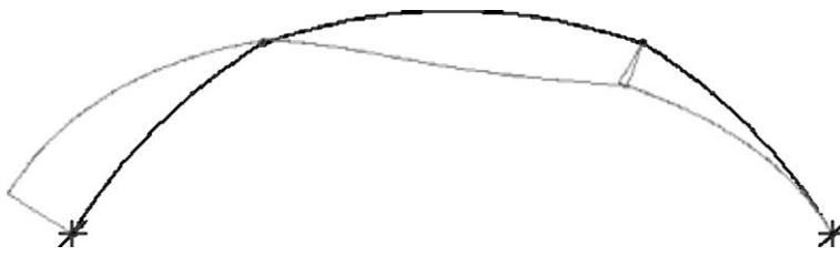
Fig. 7. Influence line of the shear stress at the left clamp for a vertical moving force.
