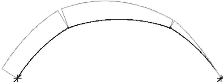
Fig. 8. Influence line of the normal stress at the left clamp for a vertical moving force.
