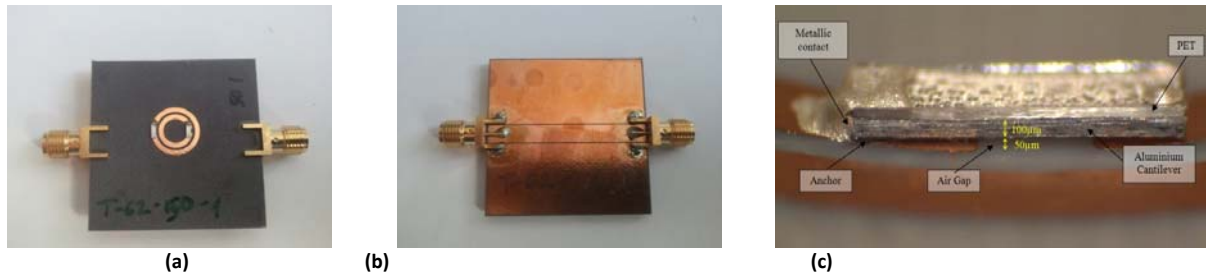
Figure 3 : passive EM temperature-sensing prototype based on split-ring resonators : (a) split-ring resonators loaded by micro-bimorph cantilevers; (b) Coplanar Waveguide for EM excitation of the split-ring resonators and (c) Aluminium/PolyEthylene Terephthalate (PET) bimorph cantilever under microscope with PET anchor of 50 \mu\text{m} thick
