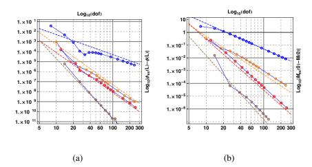
Figure 4: Figure-4(a) error's convergence for the free end rotation  $\phi(L)$ , Figure-4(b) error's convergence for the bending moment at the constrained end, for  $R/h_n = 100$  (p=2 green, p=3 blue, p=4 orange, p=5 red, and p=6 brown, p is the polynomial degree).
