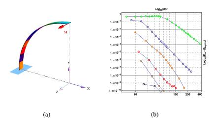
Figure 6: 3D cantilever arch with a couple at the end; 6(a) initial geometry, 6(b) convergence's error in energy, for  $R/h_n = 100$  (p=2 green, p=3 blue, p=4 orange, p=5 red, p=6 brown and p=7 black, p is the polynomial degree).
