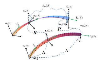
Figure 1: Intrinsic reference axes on the initial geometry of the rod
