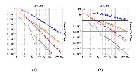
Figure 5: Figure-5(a) error's convergence for the twisting moment at the constrained end, Figure-5(b) error's convergence for the shear force at the constrained end, for  $R/h_n = 100$  (p=2 green, p=3 blue, p=4 orange, p=5 red, and p=6 brown, p is the polynomial degree).
