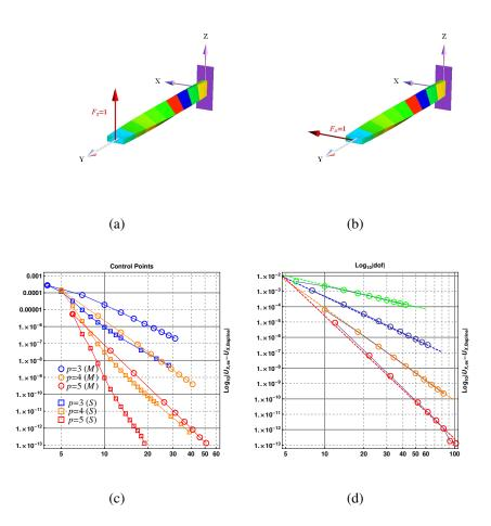
Figure 2: 3D cantilever pre-twisted beam; 2(a) initial geometry load case-1;2(b) initial geometry load case-2; 2(c) convergence's error for the  $u_z(L)$  at the free end; 2(d) convergence's error for the  $u_x(L)$  at the free end (p=2 green, p=3 blue, p=4 orange, and p=5 red, p is the polynomial degree).
