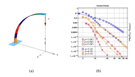
Figure 8: 2D cantilever arch with a point force at the end; 8(a) initial geometry, 8(b) convergence's error in energy, for  $R/h_n = 100$  (p=3 blue, p=4 orange and p=5 red p is the polynomial degree); the  $\bigcirc$ -markers for the  $G^1$ -multipatch and the  $\square$ -marker for the h-refinement analysis.
