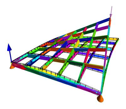
Figure 12: Initial and deformed configurations of the hyperboloid Kirchhoff-Love grid.
