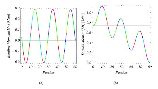
Figure 11: Stress resultant for the helix; 11(a) Bending moment; 11(b) Twisting moment.
