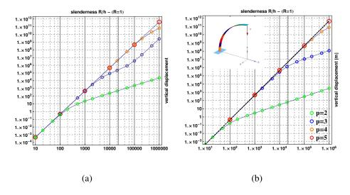
Figure 9: Influence of the slenderness ratio on the vertical displacement of the free end;  $9(a) G^1$ -mulipatch analysis; 9(b) h-refinement in single B-Spline patch; (p=2 green, p=3 blue, p=4 orange, p=5 red, p is the polynomial degree).
