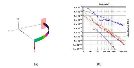
Figure 3: 3D cantilever arch with a point force at the end; 3(a) initial geometry, 3(b) convergence's error for the vertical displacement at the free end  $u_z(L)$ , for  $R/h_n = 100$  (p=2 green, p=3 blue, p=4 orange, p=5 red, and p=6 brown, p is the polynomial degree).
