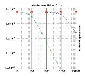
Figure 7: Influence of the slenderness ratio on the vertical displacement of the free end, (p=2 green, p=3 blue, p=4 orange, p=5 red, p is the polynomial degree).
