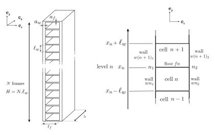
Fig. 2 The class of studied structures (left) and the basic frame and notations (right)
