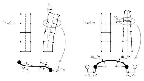
Fig. 3 Decoupling of transverse (left) and longitudinal (right) kinematics
