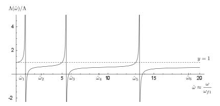
Fig. 7 Effect of the local resonance on the apparent dimensionless mass  $\Lambda(\hat{\omega})/\Lambda$  for  $\Lambda_w = \Lambda_f$
