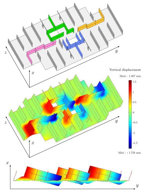
Fig. 12 Finite element modeling of one story for the calculation of the shear rigidity of the cell K in direction y. Top: undeformed story, middle and bottom: deformed story.
