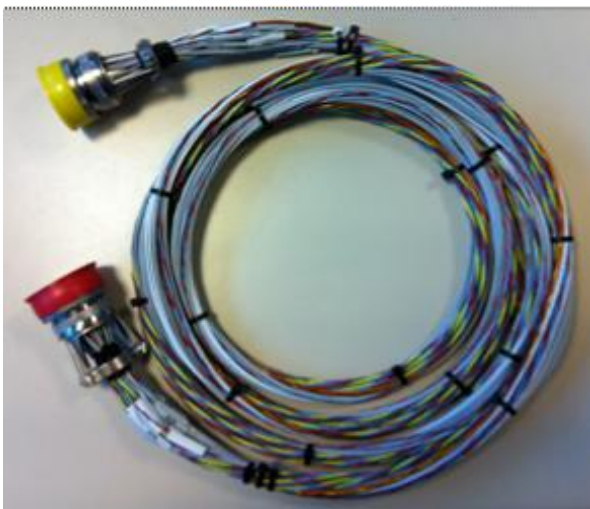
Figure 1. Picture of the complex bundle composed of 58 cables
