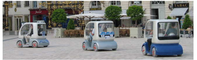
Fig. 7. Cooperative cybercars in the French city of Nancy during the MobiVIP project: INRIA develops fully automated transportation systems that need cooperative motion planning (here is a platooning example).
