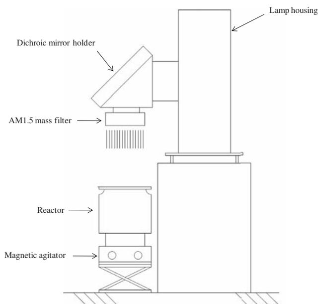
**Fig. 1 – Photocatalytic reactor.**
