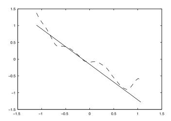
FIGURE 4. Drift's estimation for the Duffing oscillator: theoretical  $g(x_0, \cdot)$  in plain line, estimated in dashed line for  $x_0 = -0.0498$
