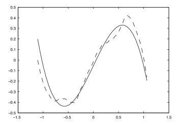
FIGURE 3. Drift's estimation for the Duffing oscillator: theoretical  $g(\cdot, y_0)$  in plain line, estimated in dashed line for  $y_0 = 0.0533$
