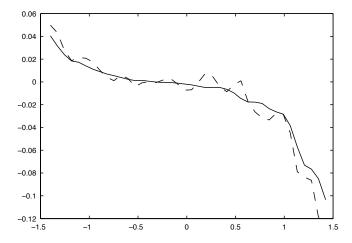
FIGURE 5. Drift's estimation for the Van der Pol oscillator: theoretical  $g(\cdot,y_0)*p_s(\cdot,y_0)$  in plain line, estimated in dashed line for  $y_0=0.0597$
