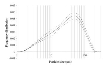
Fig. 2. Distribution of mass fractions  $f_i$  with their 95% confidence interval estimated from analysis of 13 hydrocyclone feed size distribution samples.
