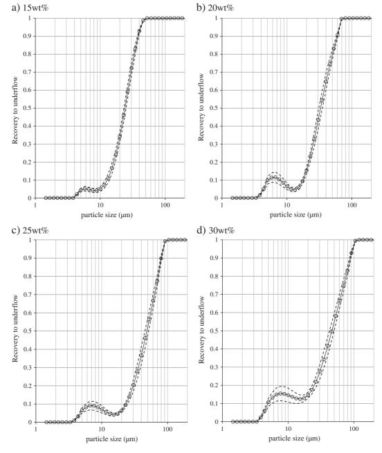
Fig. 7. Estimated partition functions for a 100 mm diameter hydrocyclone with feed solids concentration in the range 15 wt.% to 50 wt.% in 5 wt.% increments.
