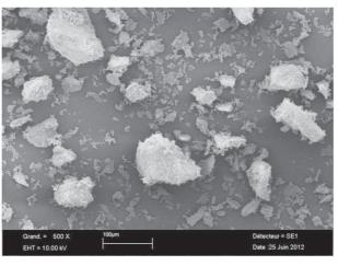
Fig. 3. SEM photomicrographs of silica particles.
