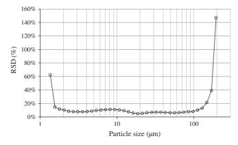
Fig. 4. RSD (%) values for particle size distribution assays  $f_i^{\prime}$  in all the measured size classes.
