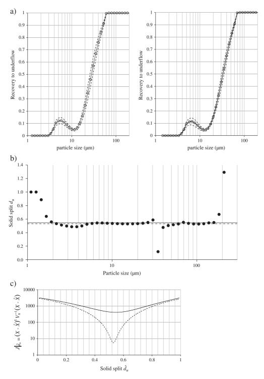
$\textbf{Fig. 6.} \ \ \text{Comparison between the mass balancing outputs using the average RSD of 8.415\% and the size-dependent RSD.}$
