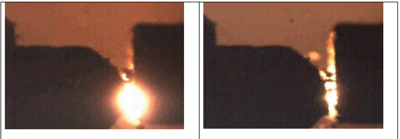
Figs. 10a and 10b. Still photographs taken from video 3 in the supplemental material showing the presence of solid carbon bridges formed by arc damage to the electrodes that present excellent triggers for further arcing.
