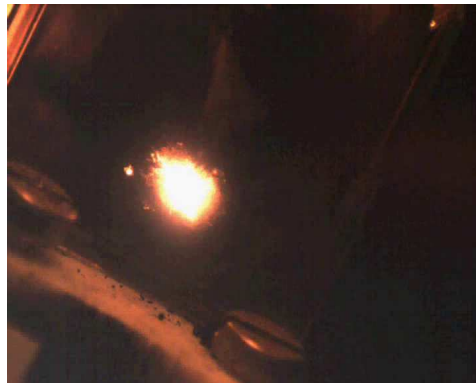
Fig. 2: Glowing pockets of hot carbon within the insulation of a damaged two-wire cable that lead to arc re-ignition. Picture taken from a slow motion video (Supplemental material, video 2).
