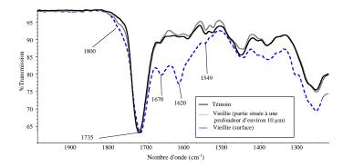
Figure 25.4. IRTF spectra in ATR mode for the surface coats of urethane-alkyd paint witnesses, aged naturally over 12 months in Florida, and located at a depth of approximately 10 μm of the aged paint
