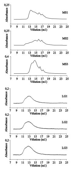
Figure 25.5. Chromatograms of commercial PNS and PMS
