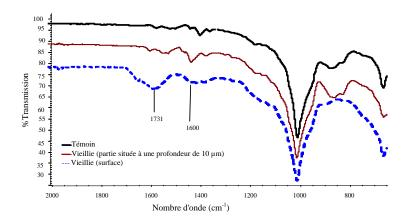
Figure 25.3. IRTF spectra in ATR mode, the surface parts of chlorinated rubber paint, aged naturally for 12 months in Florida, and the part located at a depth of approximately 10 µm in the aged system
