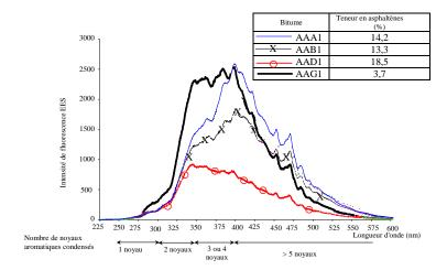
Figure 25.1. Ultraviolet fluorescence spectroscopy (UVFS) in excitation-emission matrix spectroscopy (EEMS) of four bitumens from the SHRP
